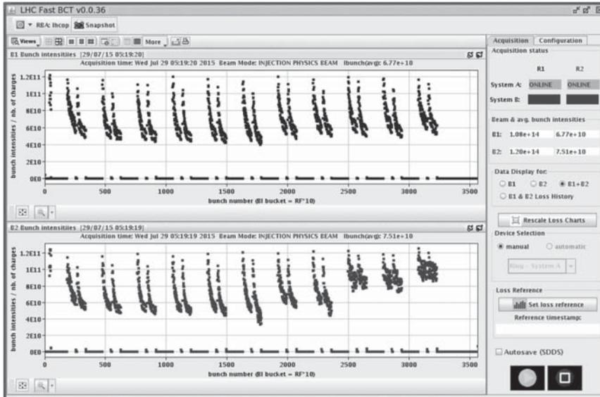
**Figure 8.26** A typical signature of electron cloud observed on a bunch intensity fixed display of the CERN Large Hadron Collider (fill 4088, 29 July 2015).
