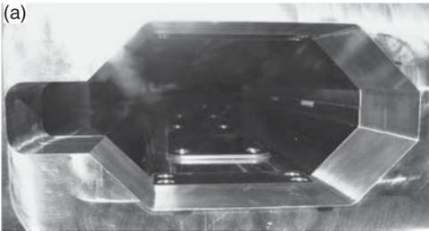
**Figure 8.14** (a) Clearing electrode in a DAΦNE dipole vacuum chamber. (b) Electron intensity grow rate. Source: Wang et al. 2006 [89], Figs. 5 and 14. Reprinted with permission of Creative Commons Attribution 3.0 license (CC-BY 3.0).
